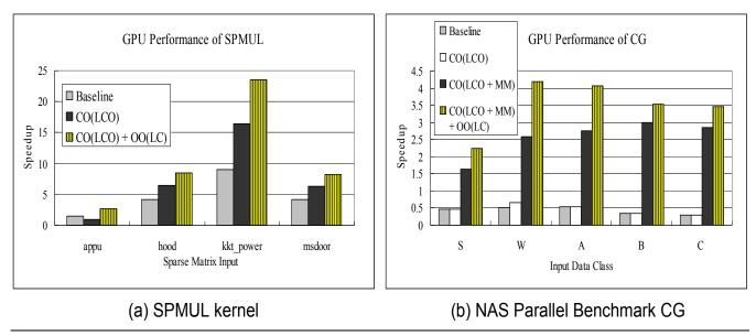
**Figure 7.** Performance of Irregular Applications (speedups are over serial on the CPU). *Baseline* is the baseline translation without optimization; the other bars represent the following OpenMP optimizations (*OO*) or CUDA optimizations (*CO*): *LCO* is a local caching optimization for global data, *LC* means the *loop collapsing* transformation technique, and *MM* represents a redundant memory transfer minimizing optimization.
